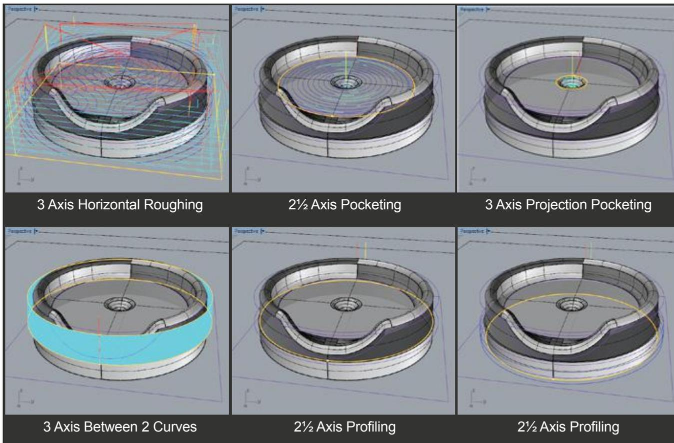
Here are the toolpaths in Setup 2 that Gordon has programmed using a 12.7 (½”) ball mill:
