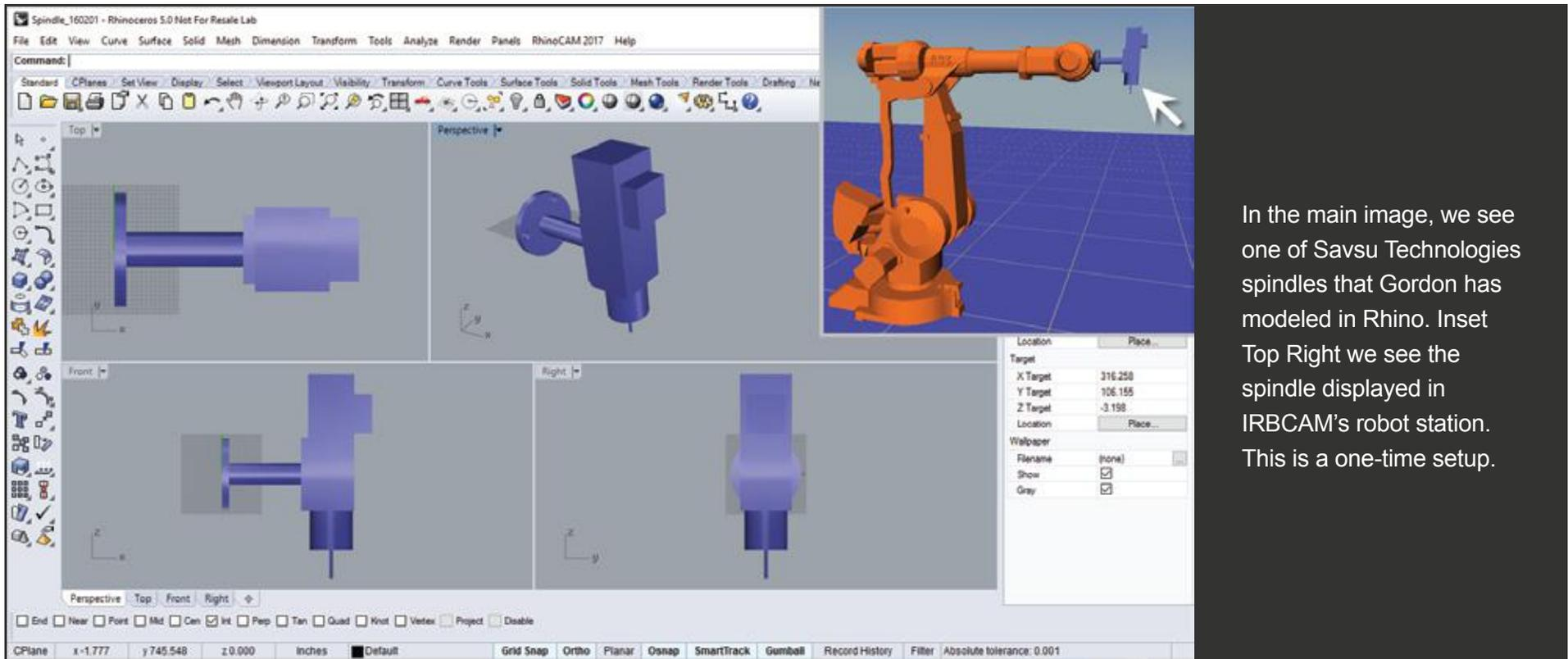
In the main image, we see one of Savsu Technologies spindles that Gordon has modeled in Rhino. Inset Top Right we see the spindle displayed in IRBCAM's robot station. This is a one-time setup.
