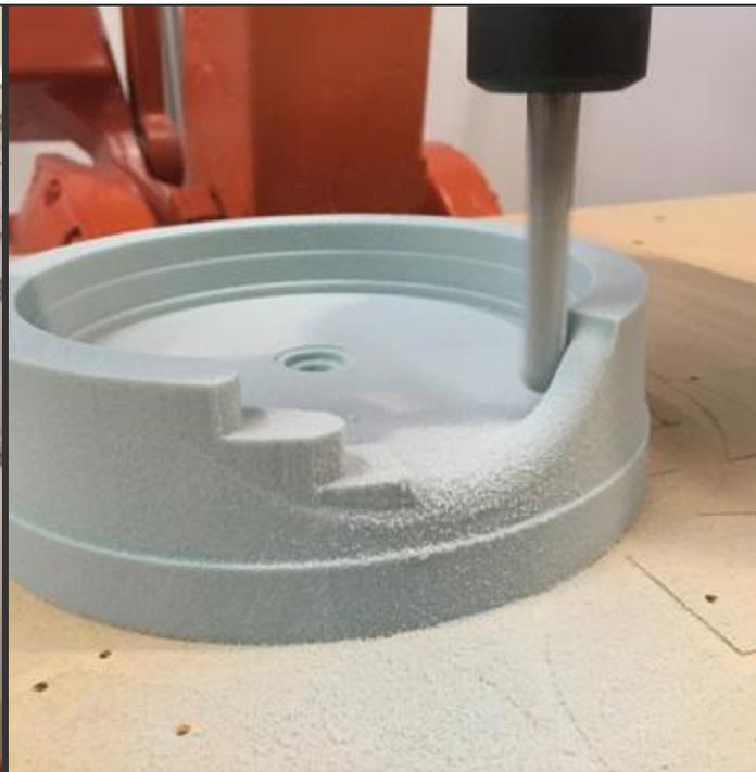
Using RhinoCAM and IRBCAM, Savsu engineers can have a design review in the morning and physical prototypes for testing in the afternoon. That's Rapid Prototyping at its finest!
